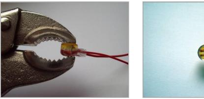
Test all connections after crimping to ensure continuity and security of connections.
