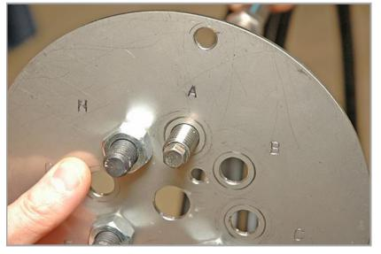
Refit the securing nut and tighten into position using the 22mm socket while holding the head tube by the anti rotation nut with the 22mm spanner
