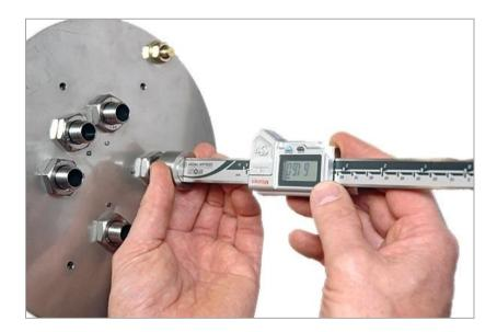
Slide the display towards the boss until the contact rests on the reading datum and record the reading that is show on the display along with the anchor position.
