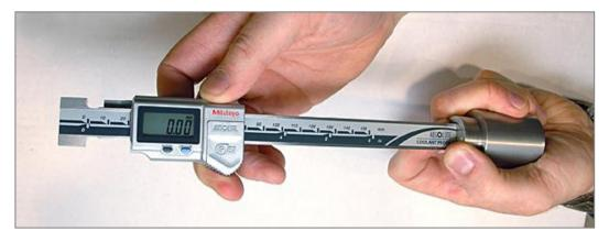
Hold the gauge boss tight into the reference block and move the digital display towards the reference block until the contact rests on the datum point.
