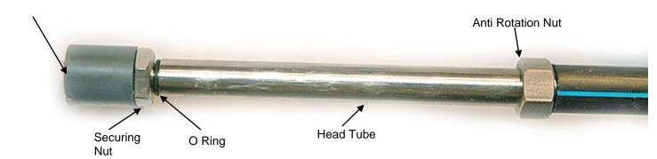
To fit the anchor head tube to the grout plate remove the protective cap and securing nut from the head tube and lubricate the "O" ring with silicon grease.
