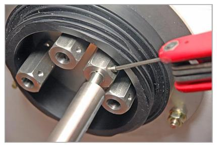
Insert the clamp screw into the clamp bush screw hole and tighten only sufficiently to ensure the collet is retained.
