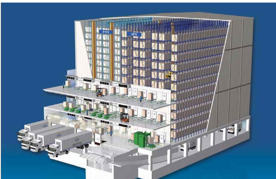
AUTOMATIC STORAGE AND RETRIVAL SYSTEM (AS/RS)
