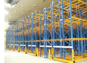
Aisle saver pallet rack with most utilization of space
