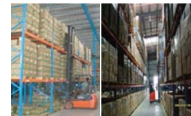
Aisle saver pallet rack with most utilization of space
