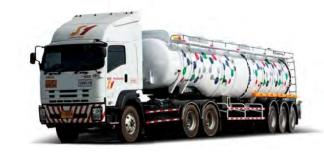
• Petroleum tankers (16-48 C.U.M.) (for truck and semi-trailer)(Carbon steel and Aluminium Alloy) standard ADR/TPII
