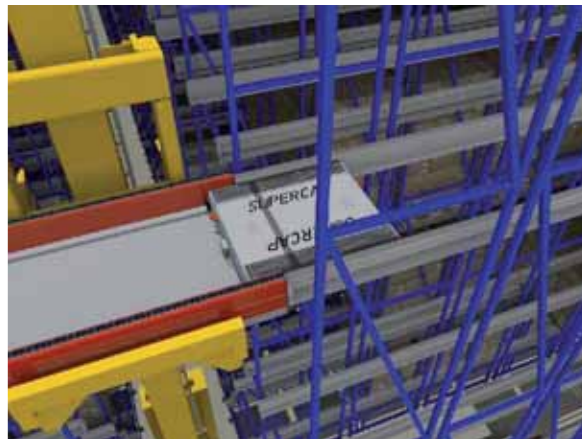
• RENDERING SHOWING SUPERCAP CHARGING PROCESS ON BOARD THE STACKER CRANE CRADLE
