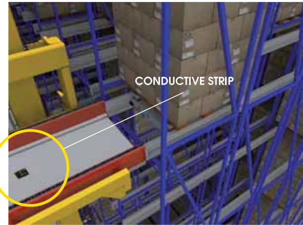
• RENDERING SHOWING THE SUPERCAP WORKING ON BOARD A STACKER CRANE
