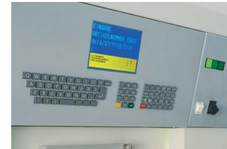
Keyboard in the Rotomat control box above the retrieval point, keys positioned centrally at eye level (standard)
