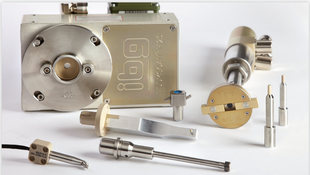
Highest test reliability and sensitivity - different kinds of probes for crack and grinder burn detection. Back left a rotating head eddyscan H for testing a string of parts and bars, back right a rotating head eddyscan F for testing of boreholes and surfaces.
