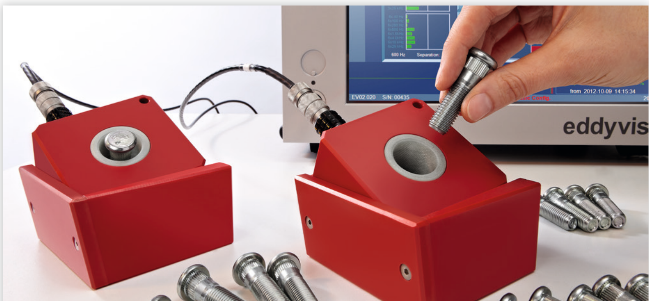
Fixture for manual eddy current structure test in the lab.
