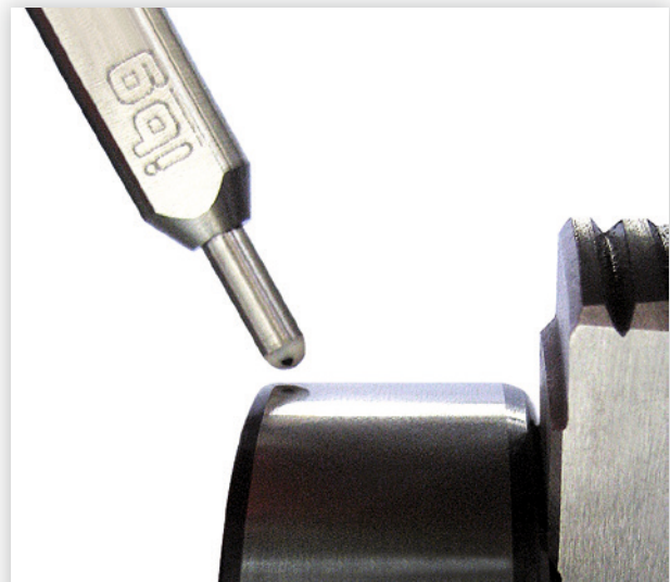
Crack and grinder burn detection on a bearing ring using a spherical X-type differential probe manufactured by ibg.
