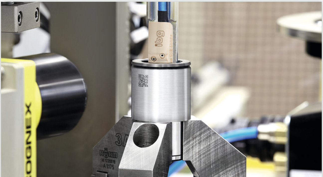
Steering nut in an automatic ibg test system. Detection of cracks and grinder burn defects on the race inside. With camera inspection system to capture part type specific QR-code.
