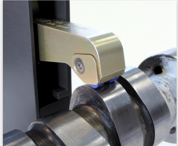
Crack detection probe box for contacting testing on eccentric parts like camshaft lobes for cracks and grinder burn; large diameter range is covered; up to 300 rpm (depending of part geometry), ceramic supports for long life-time. Solutions for structure test on camshafts on request.
