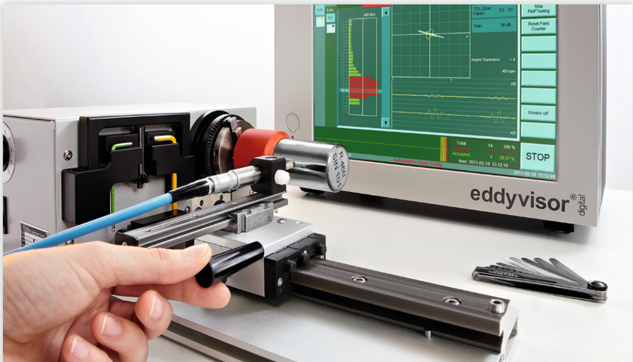
ibg lathe for lab tests, feasibility studies and small series in crack detection with eddyvisor. Speed max. 850 rpm, chuck up to 68 mm diameter, with trigger sensor, flexible probe movement.
