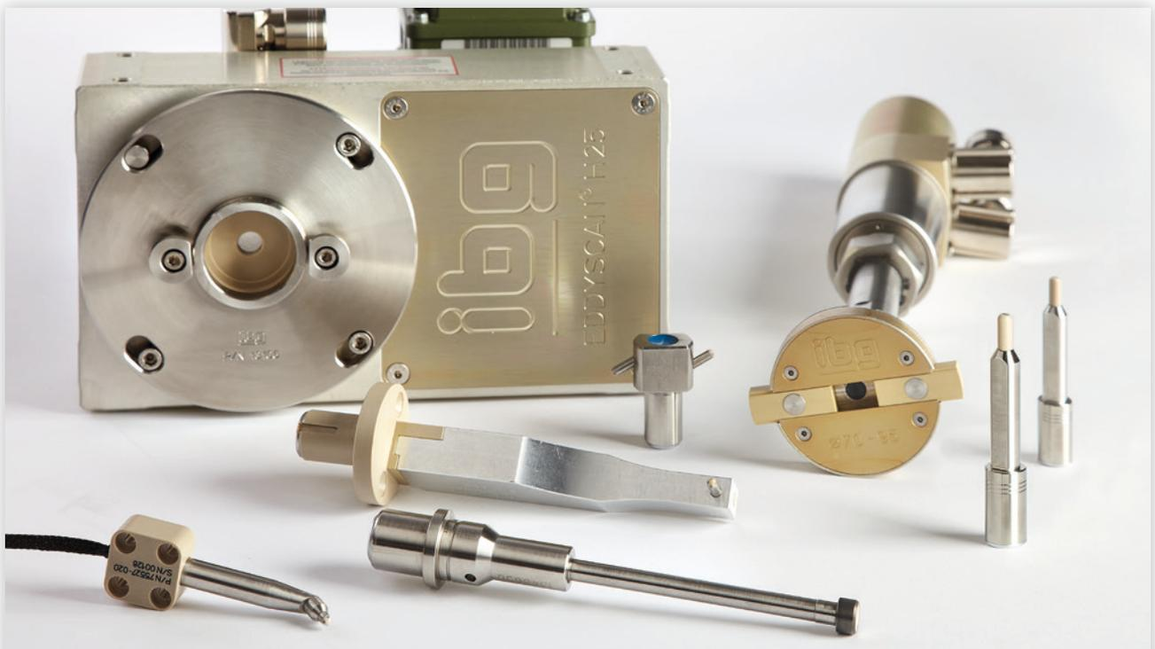
High testing accuracy, sensitivity and temperature stability - probes of different design for crack and grinder burn detection. Back-left an eddyscan H rotating head for testing parts in a line. Back-right an eddyscan F for testing boreholes and surfaces.
