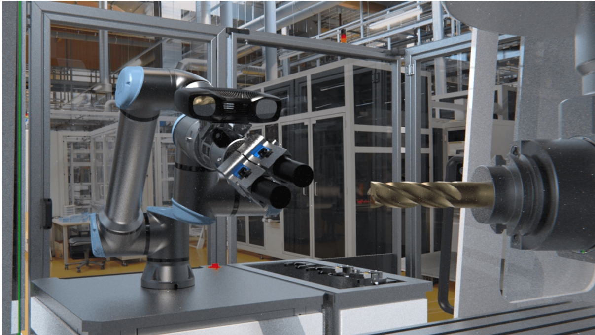
A Zivid Two 3D camera mounted on a robot arm for machine tending.
