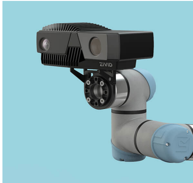
Example of Zivid's on-arm mount with a 3D camera on Universal Robots.
