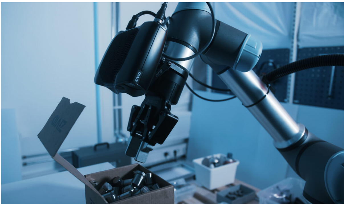
A robot-mounted camera can get close to target objects.
