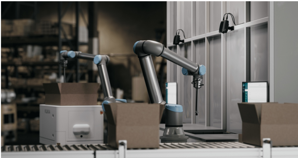
Stationary mounted Zivid Two 3D cameras in manufacturing
