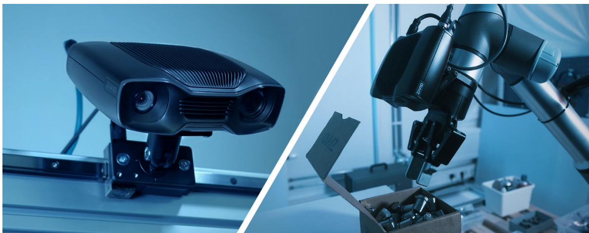
Stationary mounting (left) vs. on-arm mounting (right) with a Zivid Two 3D camera
