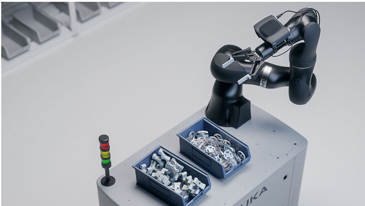
A robot mounted Zivid Two 3D camera for bin-picking
