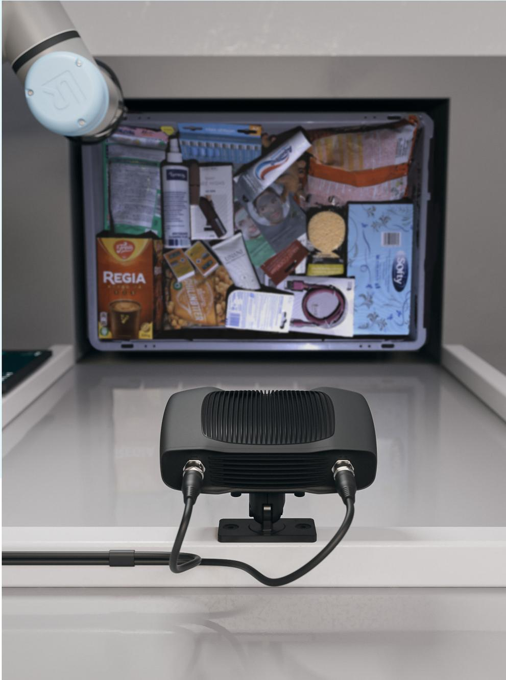
**Robotic piece picking** is the process of automated order fulfillment, picking various individual items (SKUs) from an inventory bin and place them in an order container for shipping to customers. The choice of the vision system and, in particular, the 3D camera impacts the robot's ability to successfully detect, pick, and place all types of pieces.
