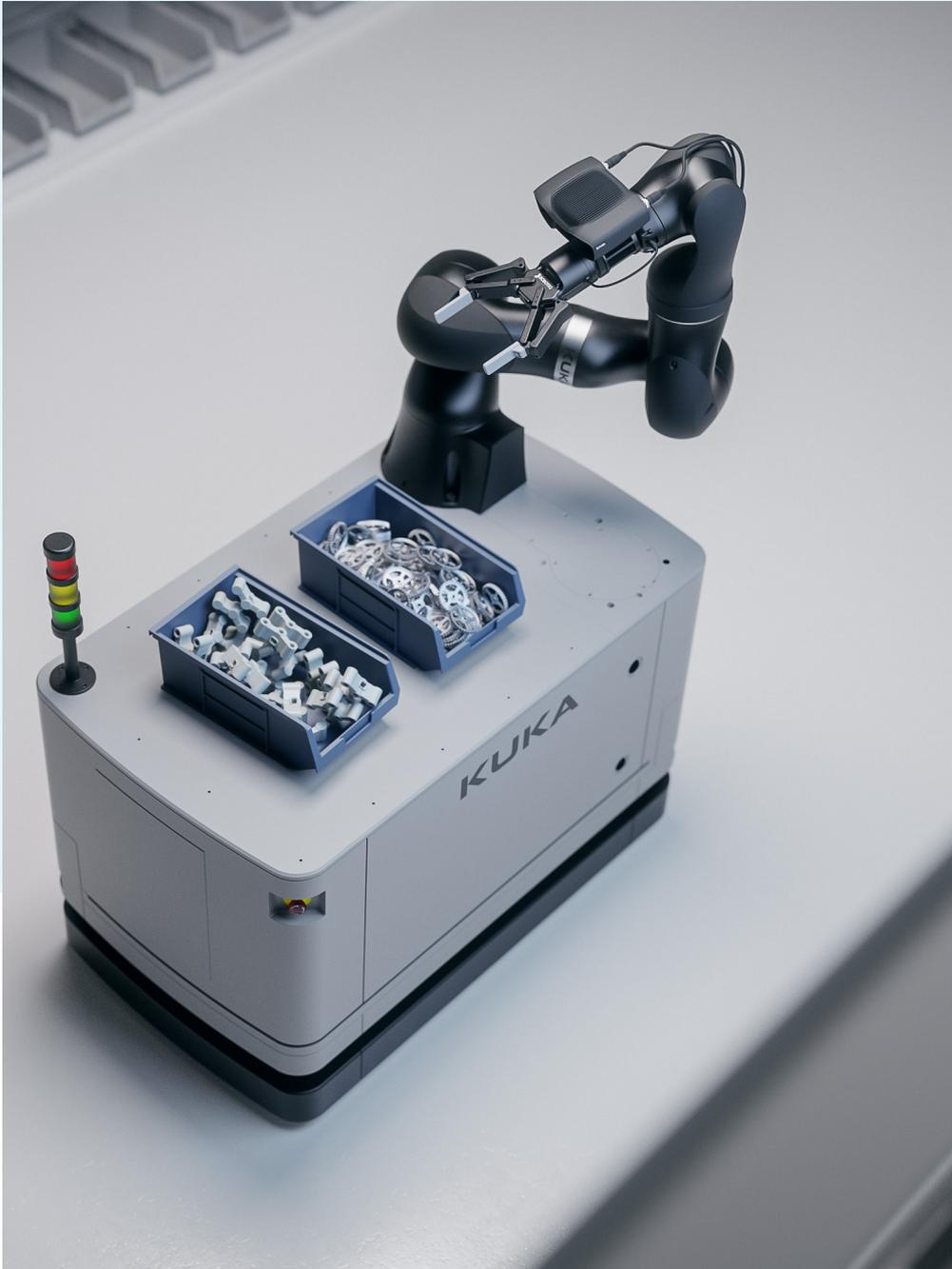
**Random bin picking** is typically at the input stage of a manufacturing process. Instead of traditional static fixtures or pre-filled stacking patterns, a robot is instead emptying a bin bulk-filled with parts for placing on, for example, a feeder, conveyor, or sorter for further processing in the plant. The choice of the vision system and, in particular, the 3D camera impacts the robot's ability to successfully detect, pick, and place all types of parts.
