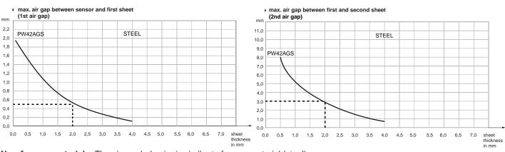
Non-ferrous materials: The air gap behavior is similar to ferrous material (steel).
