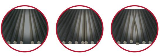
Reliable detection of material faults in steel cord: open splice or missing wire (left) double or narrow wires (middle) and locale defects, such as crossed, loose or jumped wires (right).
