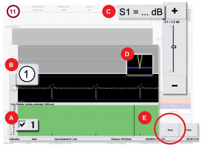
11. Select the sensor for calibration (A), click on sensor button (B), adjust gain value for the selected sensor (C); each signal of the Missing Wire (MW) signal (D) must reach the negative threshold.
