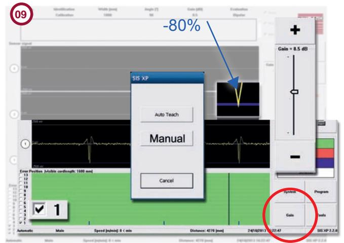
09. Run the conveyor belt and start the machine. Select sensor 1 and deactivate all others. Change **Gain** till Missing Wire (MW) reaches -80% threshold.
