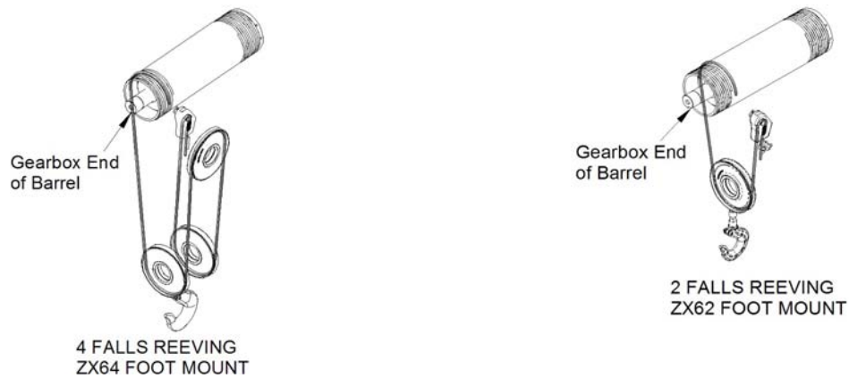
Figure 64 – Reeling Diagrams for Foot Mount Hoists: ZX062-FTM / ZX064-FTM
