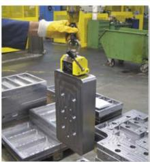
Loads with limited contact surfaces can be safely handled and the deposit area can be optimized.
