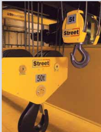
Main and auxiliary hoist
