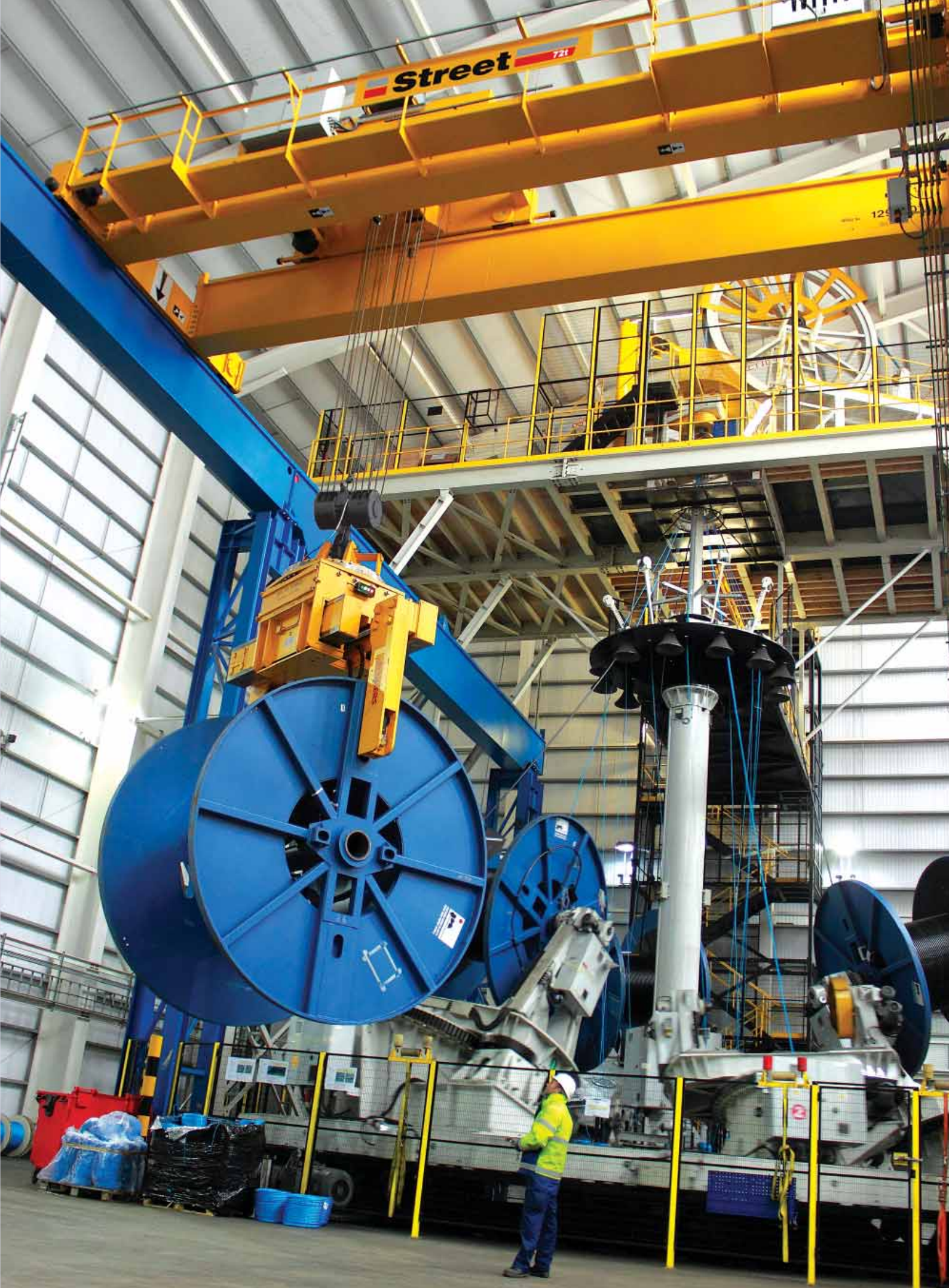
72t crane with grab
