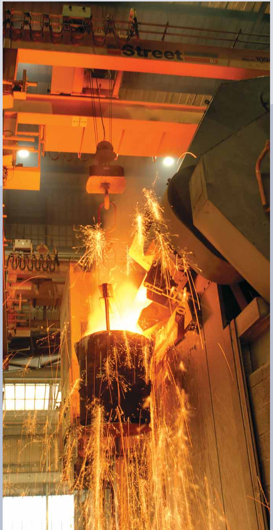
Hot metal ladle crane
