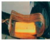
300 × 300 × 600mm 鋼板加熱 Heating steel plate
