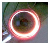
齒輪淬火 Quenching gear
