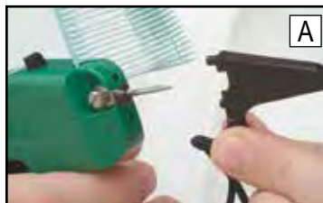
A safety cover provided to snap over the injector needle when not in use.
