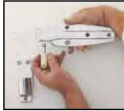
Pop out cap. Turn strap 180°, reinsert pin in strap.
