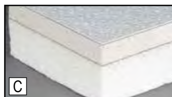
C. 1-inch EPS Foam is laminated to 1/2-inch fire and moisture-resistant gypsum and FiberLite FRP one side only. 2 feet x 4 feet.
