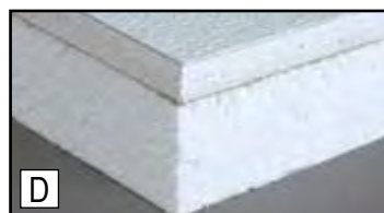
D. 1 1/2-inch EPS Foam is laminated to 1/2-inch fire and moisture-resistant gypsum and FiberLite FRP one side only. 2 feet x 4 feet.
