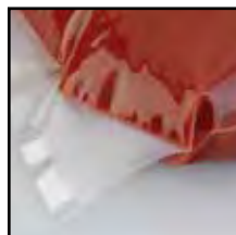
On larger bags an angled seal adds extra strength and a surface to hold onto.
