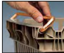
Two 3/8 inch zinc-plated steel wire bails swing down to allow nesting and swing up for stacking.
