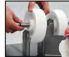
Replaceable wheels and bushings.
