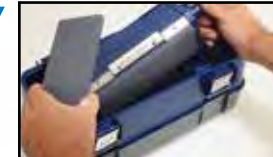
Stones are changed individually and locked into place.
