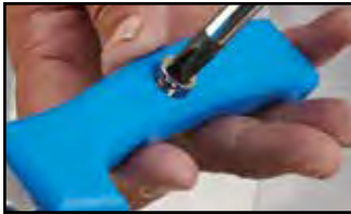
Remove screw and the double-bladed knife becomes two separate knives.
