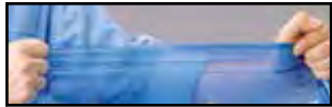
4 mil VR is comparable to 6 mil PVC. 6 mil VR is equivalent to 8 mil PVC.
