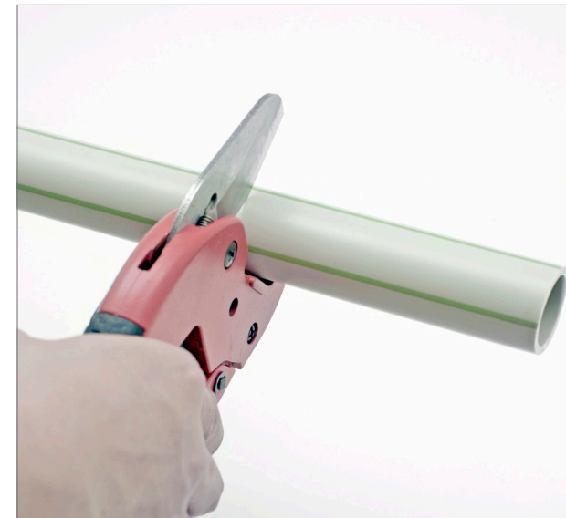
Cut the pipes
