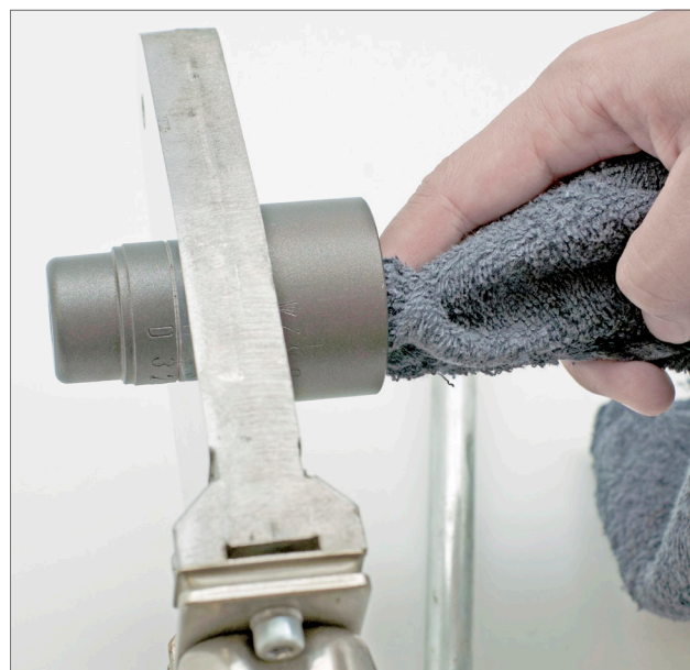
Clean the heating bushes
