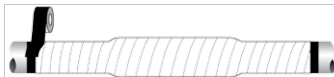
Fig. 21-12 Wrapping the protection area with black/grey tape
