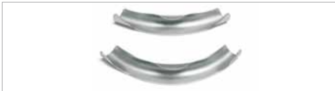
Fig. 13-2 Pipe bend bracket for plumbing (5 x d), 90° and 45° for sizes 16 – 25
