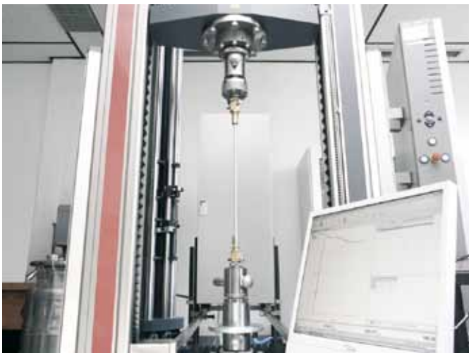
Fig. 4-7 Procedure of a tensile test
