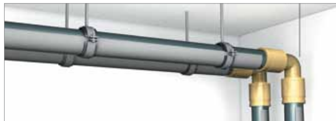
Fig. 14-3 Maximum pipe clamp intervals
