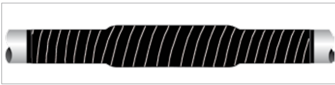
Fig. 21-13 Fully protected joint with corrosion protection system.
