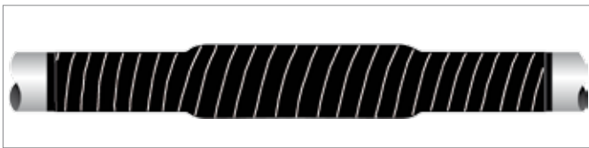
Fig. 21-13 Fully protected joint with corrosion protection system.
