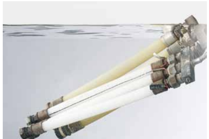
Fig. 4-8 Pipes in a long-term test (under pressure in a water bath)
