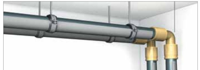
Fig. 14-3 Maximum pipe clamp intervals
