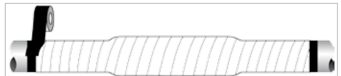
Fig. 21-12 Wrapping the protection area with black/grey tape
