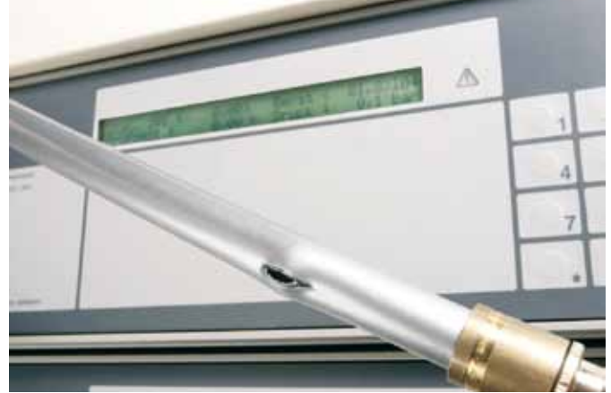
Fig. 4-5 Result of a burst pressure test with the universal pipe RAUTITAN flex
