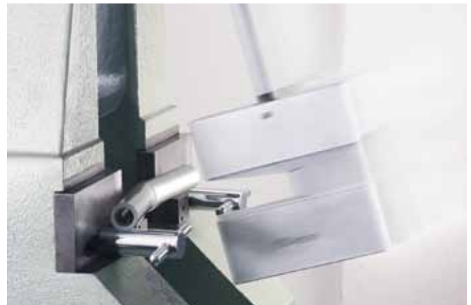
Fig. 4-6 Universal pipe RAUTITAN flex in the notch impact testing device
