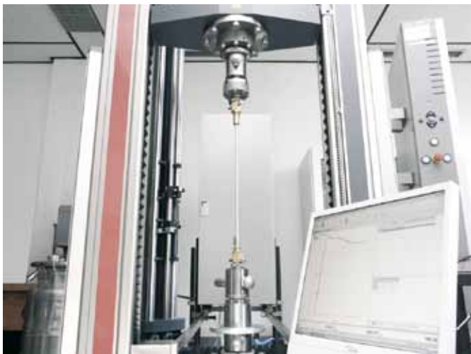
Fig. 4-7 Procedure of a tensile test
