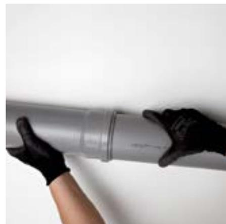
A system that is suitable for temperature fluctuations: **the thermal expansion of Valsir PP3® is extremely low compared to the most common plastic materials**, a 3 m pipe will expand in length by just 13 mm when the waste liquid flows at a continuous temperature of 60°C.
