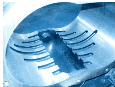
Pulse Eraser (pressure pulsation reduction mechanism)
