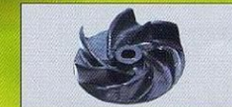
Impeller made of engineering plastic After 200 hours of pump operation Loss of impeller weight: 3.3%
