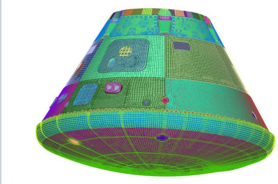
From advanced beam modeling, mid-surface extraction and hex meshing to robust CAD import and idealization, Femap gives you unparalleled model control and flexibility with a broad range of loads, materials, analysis types and visualization options.
