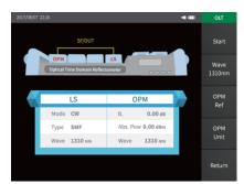
Combining module light source with the Power Meter supports use as a Loss Test Set.
