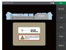
The VFL, available as a standard module in NOV6800 series OTDR, offers built-in 650nm visual fault location on a FC/UPC connector.
