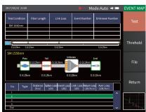
NOV6800 series OTDR uses 1625nm wavelength to scan and analyze the access point and proceed online testing with optical filter and will not disturb the service. It could pass the 1:  $2 \sim 1$ : 64 optical splitter
