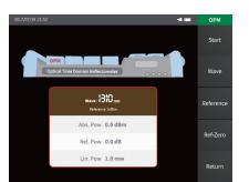
NOV6800 series OTDR comes with optional built-in power meter that let technicians easily verify the presence of a signal
