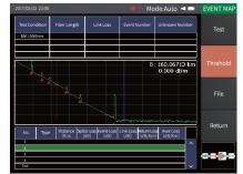
OTDR mode allows for measuring distance, loss, reflectivity, attenuation and accumulation loss on a fiber optic link.
