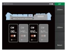
NOV6800 series OTDR comes with optional built-in laser source through OTDR Port that let technicians easily verify the total loss of the local network with a power meter.
