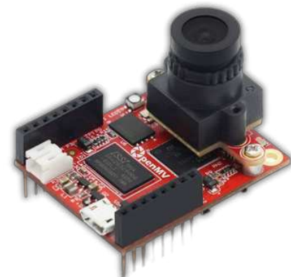
OpenMV Cam H7 Plus microcontroller board with high Resolution Cam
