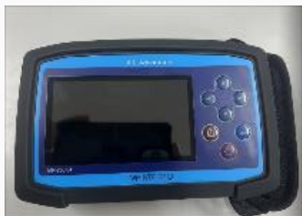
Air Leaks Thermal Scanner
