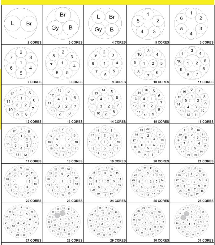
NOTE: Fillers are necessary to fill the cable a substantially circular cross section.
