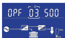
Frequency Setting (50 or 60Hz)
