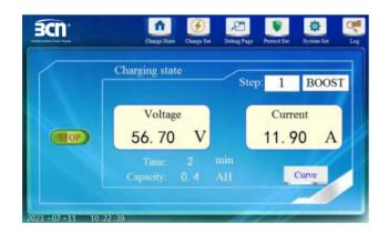
The display and operation unit mounted on the front door of the touch screen display to indicate the status and the measurements in plain text, as well as 11 LED controlled by the monitoring and control unit. In addition, the front panel is equipped with Boost-float change-over switch and manual-automatic change-over switch, which are used to switch charging mode; it is equipped with circuit breaker and fuse to protect the input and output of charger.
