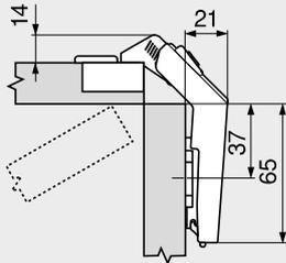
Application for 19 mm thick door in conjunction with 0 mm spaced standard mounting plate
