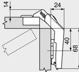
Application for 19 mm thick door in conjunction with 3 mm spaced standard mounting plate
