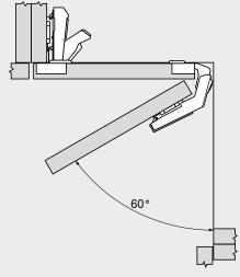
Application for 19 mm thick door in conjunction with 0 mm spaced standard mounting plate
