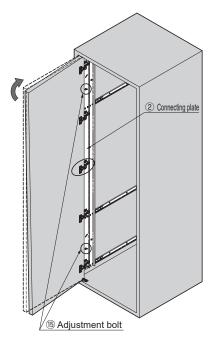
Check that the screws fixing the connecting plate and the adjustment bolts are loose.
