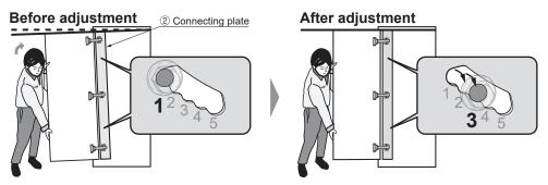
3 Tighten all the temporarily fastened screws.
