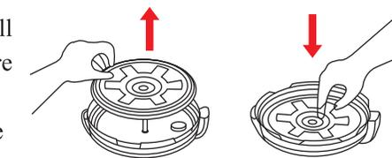
Clean up the pressure limited valve : Pull the pressure limited valve to clean up then installed back to the properly position.
