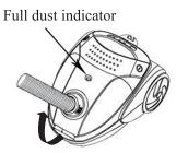
1. Press the locking block to open the front cover.
