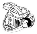
4. When the motor filter is dirty remove the filter and wash carefully in liquid or water. Allow the filter to dry completely before replacing it.
