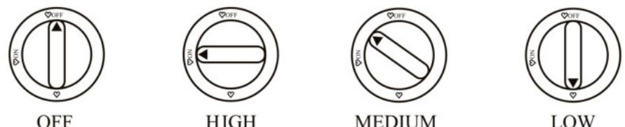
7. Fire off, turn the knob clockwise to the “OFF” position and hear a “ta” at this time, the air path is cut off, the fire in the oven went out.
