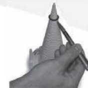
Identification of the 2-xxx size number with the measuring cone
