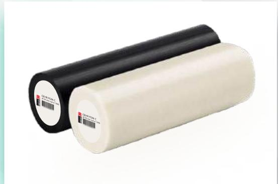
The continuous operating temperature of polyoxymethylene ranges between -40°C and +100°C. The high surface strength is only surpassed by a few materials. POM shows good sliding properties and high resistance to wear and tear because of the high strength and smooth surface. There is a very low risk of stress cracks. POM-C (Copolymere) exhibits a high thermal stability and a high resistance to chemicals (high resistance to hydrolysis).
