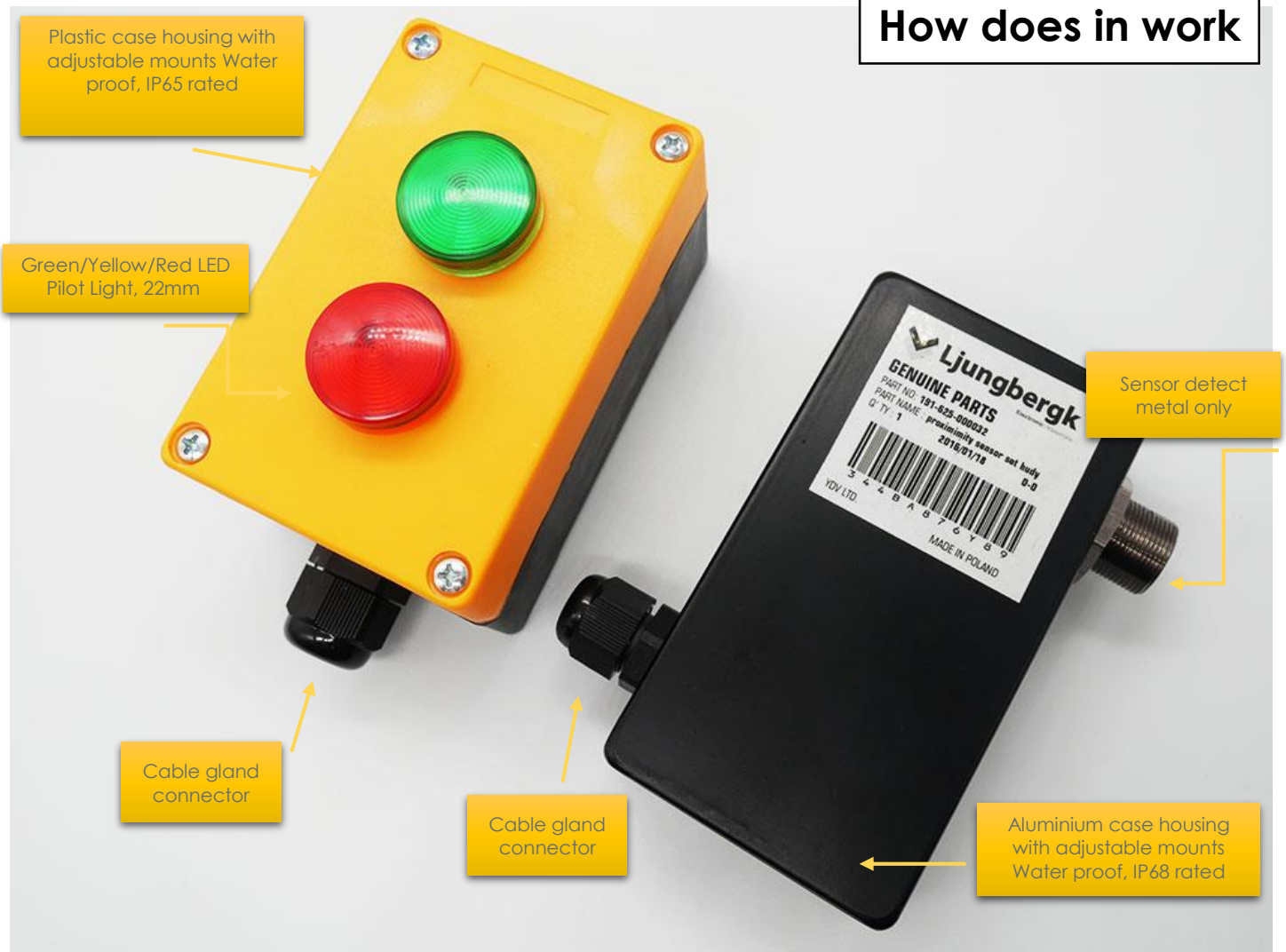
Dump truck sensor (detect metal )+ Indicator light | Buzzer Alarm
