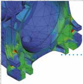
The housing has been designed with parametric three-dimensional CAD SW supported by programs of analysis of the thermal dissipation capacity and the structural resistance/deformation.
