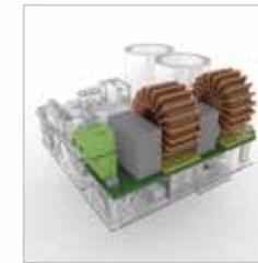
The EMC filter makes NANO compatible not just with industrial environment, but also with light industrial, commercial end residential environments.
