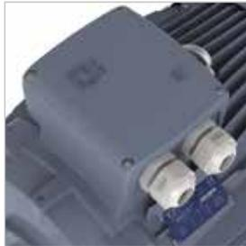
Keeping the same sealing system of the whole delphi series, the terminal box up to size 280 is made in aluminum, thus guaranteeing its IP65 protection index without being affected by the usual finishing imperfections of the cast iron
