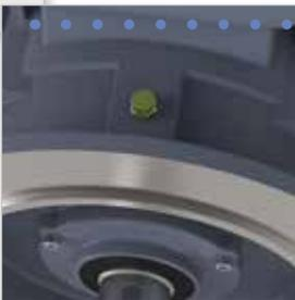
Instead, from size 315 and up, they are provided with lubricators. 4, 6 and 8 poles motors drive end bearings are in fact of open roller type, in order to withstand eventual extraordinary radial loads (see paragraph "components list")
