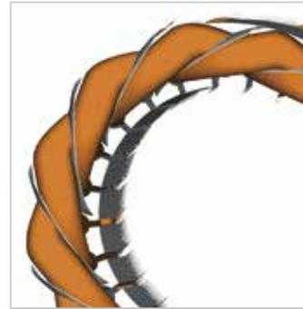
The copper is impregnated with a double layer of insulating enamel to ensure high resistance to electrical, thermal and mechanical stress. The phases are further isolated by another layer of Nomex film to protect the motors from the voltage peaks that usually occur when the motor is controlled by an inverter.
