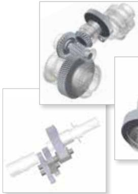
Use of high strength steels and case hardening to  $58 \pm 2$  HRC reduce the wear rate in wheels. All cylindrical gears are profile ground to Din 3962 class 6 accuracy for low noise and high efficiency.
