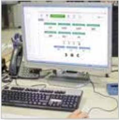
Setting and command can also be made by a PC, thanks to the free PC interface program "Motive Motor Manager"
