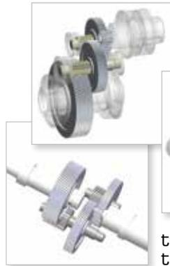
Optimal ratios (between 2 and 6) in the several stages, together with appropriate centre distances, result in higher number of teeth and size (module) of each wheel and better torque transmission fractioning through various stages.
