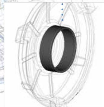
From type 90, a steel insert is provided in the bearing slot of the aluminum flanges, to resist to radial mechanical forces with a fair degree of security
