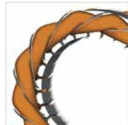
The special winding permits a good starting torque even without a double capacitor start/run
