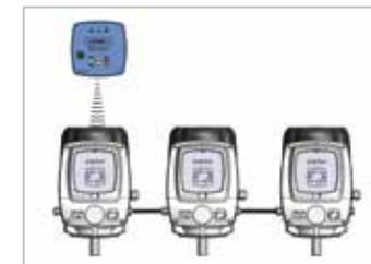
A keypad can control simultaneously, or separately, up to 8 motors.
