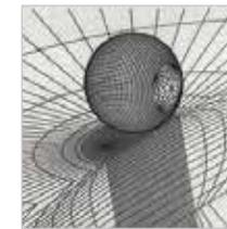
The surface is exposed to a bombardment of micro-spheres that induces compression and increases further the fatigue resistance.
