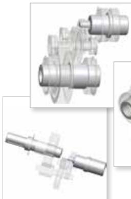
Shafts are made from 42CrMo4 steel and tempered to reach a hardness of 23-35 HRC, thus increasing their capacity to withstand shearing stresses and torsion effect.
