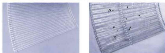
Example of a standard RA radius belt with a link at both sides, and if needed equipped with reinforcing bars
