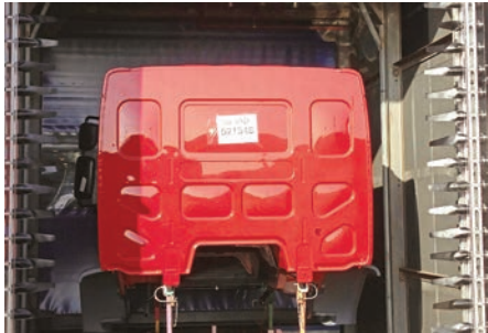
Drying truck cabs
