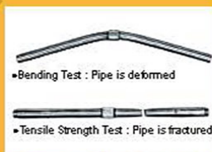
Fig. 5 In strength tests, there was no effect on the thread. The pipe itself became deformed or fractured.
