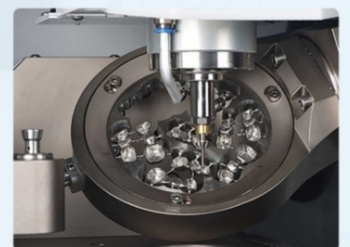
A AND B AXES CAN BE TILTED TO MILL UNDERCUTS CONTINUOUS 5 AXIS CAPABILITY OF THE MACHINE AND 5 AXIS YENADENTCAM SOFTWARE CAN DEDUCT UNDERCUTS AND MILL AUTOMATICALLY.
